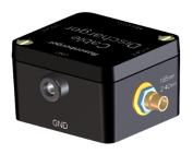
Ground the box appropriately while discharging a cable. Use the "GND" connector of the box (as shown in the figure) to the ground connector of the AXIe chassis. For grounding, either use the accessories provided with the discharger like the grounding cable or an ESD mat which is connected to the ground connector of the AXIe chassis.
